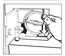
■ Pull the emergency door latch downwards (see illustration). The machine door will then open.
